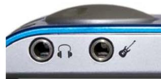
The analog outputs **Phones** (channels 3/4) are available at the breakout cable and on the right side of the unit. The connectors are not separated electrically. When connecting two headphones the volume might be reduced. The low impedance and unbalanced output signal is – in terms of quality – identical to the ones at the line outputs, but limited to +7 dBu.
