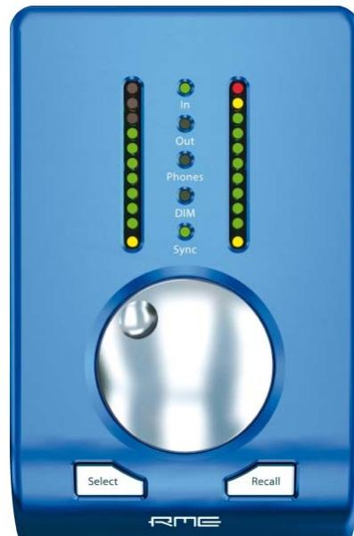
The key **Recall** is used to store and load a specific listening volume for the Main Out (default: Analog 1/2) defined in TotalMix FX. Pushing the knob for 2 seconds stores the current setting. If the volume (output level) had been changed a quick hit on the Recall key will restore the former value.
