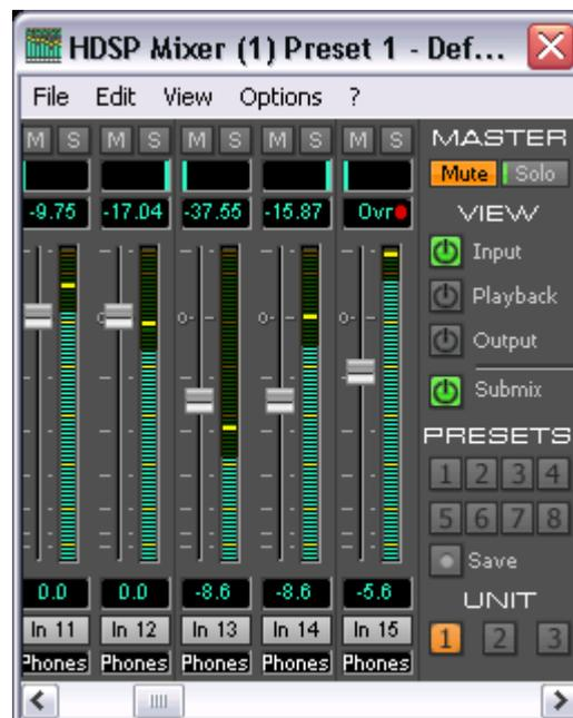
This level display of TotalMix also provides means for a constant monitoring of the signal quality. Thus it can be a valuable tool for sound optimization and error removal in the studio.
