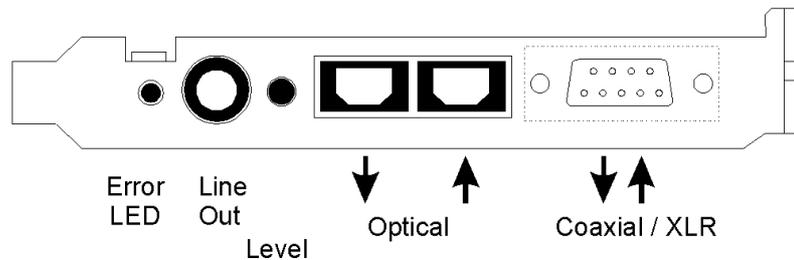
All outputs are driven in parallel, therefore carrying identical signals. In the simplest situation, connect 3 devices at the outputs and use the card as a splitter (distribution 1 to 3).
