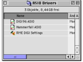
Copy the new files **RME DIGI Settings** and **Hammerfall ASIO** into all 'ASIO Drivers' folders found on your computer. As every ASIO software has its own ASIO Drivers folder the files have to be copied several times. The picture to the left shows an example after installation of Hammerfall and DIGI96.
