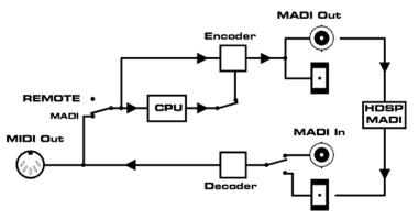
In this configuration, there is no input available for MIDI signals of external devices.
