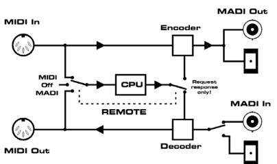
The MIDI input signal will never be transferred directly from MADI to MADI, no matter how the matrix router is set up. A MIDI cable connecting MIDI output and MIDI input of the ADI-6432, will realize a direct pass-through of MIDI, from MADI input to MADI output.
