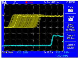
The cleaned and jitter-freed signal can be used as reference clock for any application, without any problem. The signal processed by SteadyClock is of course not only used internally, but also available at the ADI-648's word clock output. It is also used to clock the digital outputs.
