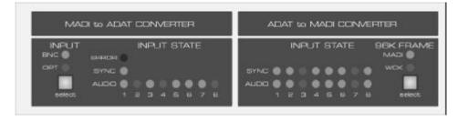
The *ADAT* to *MADI* Converter shows the Sync state for each of the 8 inputs via 8 LEDs. Again 8 LEDs display incoming audio data per 8-channel group.
