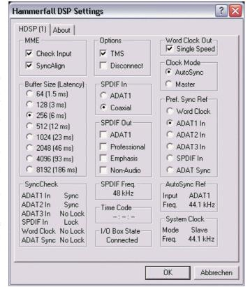
SyncCheck indicates whether there is a valid signal (Lock, No Lock) for each input (Word Clock, ADAT1-3, SPDIF, ADAT Sync), or if there is a valid *and* synchronous signal (Sync). The *AutoSync Ref*(erence) display shows the input and frequency of the current sync source.
