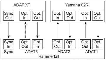
for the ADAT3 input. Because the ADAT recorder is not receiving any signals from HDSP or from the mixer, it will generate its own clock at a rate which is (almost) the same as the sample frequency of the mixing desk - but not identical.
