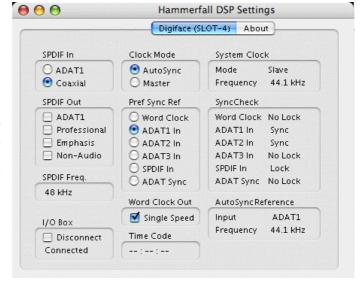
of the system, and the status of all digital signals. *SyncCheck* indicates whether there is a valid signal (Lock, No Lock) for each input (Word Clock, ADAT, SPDIF), or if there is a valid *and* synchronous signal (Sync). The *AutoSync Reference* display shows the input and frequency of the current sync source.
