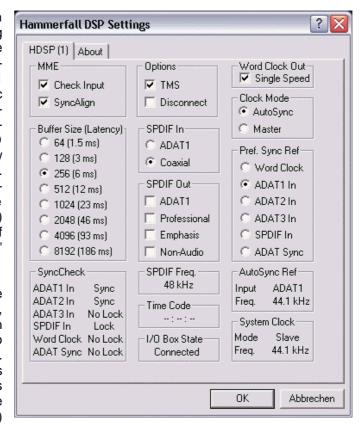
RME's exclusive **SyncCheck** technology (first implemented in the Hammerfall) enables an easy to use check and display of the current clock status. The 'SyncCheck' field indicates whether no signal ('No Lock'), a valid signal ('Lock') or a valid *and* synchronous signal ('Sync') is present at each of the digital clock source inputs. The 'AutoSync Ref' display shows the current sync source and the measured frequency.
