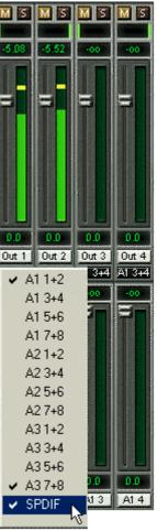
You will certainly have noticed that the signal at the outputs 7/8 did not change while you were routing channel 4 to other outputs and setting different gain values for those. With all analog and most digital mixing desks, the fader setting would affect the level for every routed bus - not so for TotalMix. TotalMix allows for setting all fader values individually. Therefore the faders and the panpots jump to the appropriate setting as soon as another routing is chosen.
