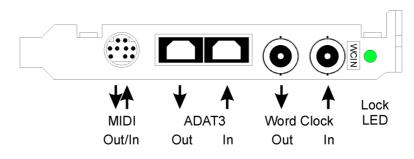
**Word Clock** I/O (BNC). When shipped, the word clock input is not terminated. Termination with 75 Ohm is available via jumper **X105** on the Expansion Board.
