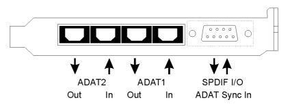
The **ADAT1** I/O next to the D-type socket can also be used as **optical SPDIF** I/O, if set up accordingly in the Settings dialog.
