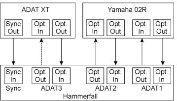
shows 'Lock' instead of 'Sync' for the ADAT3 input. Because the ADAT recorder is not receiving any signals from HDSP or from the mixer, it will generate its own clock at a rate which is (almost) the same as the sample frequency of the mixing desk - but not identical.
