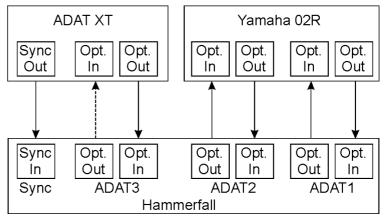
from the mixing desk), but shows 'Lock' instead of 'Sync' for the input ADAT3. Because the ADAT recorder is not receiving any signal from HDSP or from the mixer, it will generate its own clock at a rate which is (almost) the same as the sample frequency of the mixing desk - but not identical.
