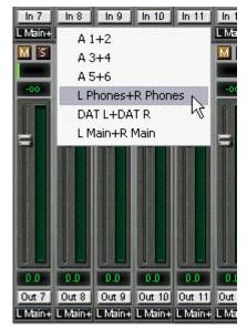
The hardware outputs (third row) can be edited in the same way. In this case, the names in the routing drop down menus will change automatically. Additionally the names in the drop down menus of the Monitor section will change as well.
