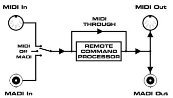
Since firmware 2.0 the Micstasy also reacts on Sysex commands from Yamaha's mixing desks M7C and PM5D. Adjustable are in this case: Input Gain in steps of 1 dB (gain range -9 up to +63 dB) and Phantom power per channel. For DM-1000 and DM-2000 see chapter 19.5.
