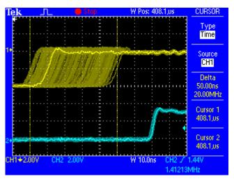
The cleaned and jitter-freed signal can be used as reference clock for any application, without any problem. The signal processed by SteadyClock is of course not only used internally, but also available at the Micstasy's word clock output. It is also used to clock the digital outputs MADI and AES/EBU.
