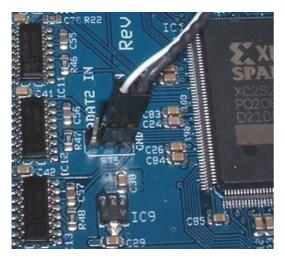
Connecting a TEB to the second ADAT In of a HDSP 9652. Remove the jumper ST5, plug DIGOUT of the TEB on both right and middle pin of ST5.
